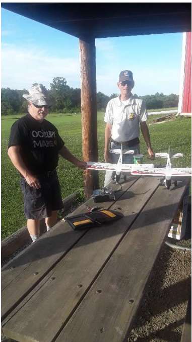
Lloyd Hinrichs and Ralph Graul with their Turbo Timber park flyers. 6 oz., 2S-300 mah lipo
