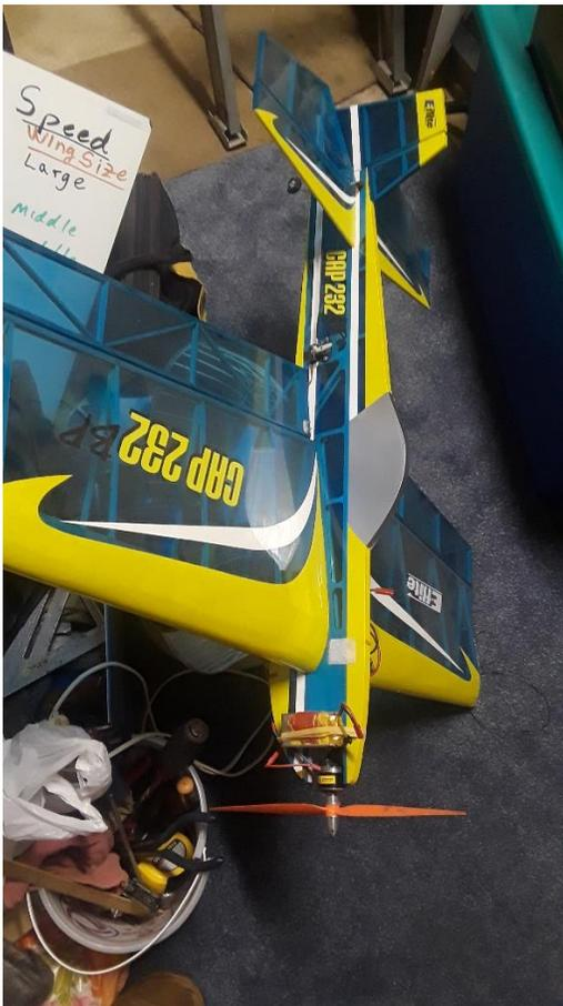
Take a look at the white square above the leading edge of the wing. This is a Velcro patch for holding the Lipo battery to the model. When I did a trial finger hold of the model at the CG with the battery attached at the square, the tail of the model hung low. Aha ! The plane was tail heavy !
