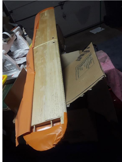
The wing's top peeled back ready for spray adhesive.
