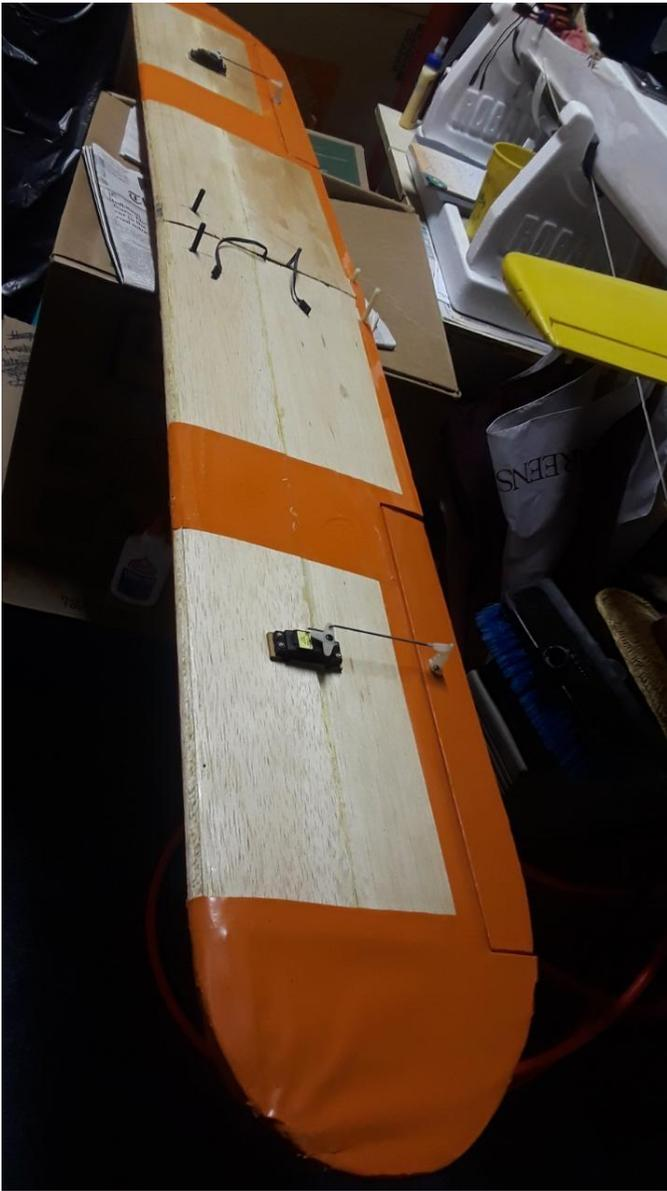
RX installation and hook up – I have an old Airtronix 72 Mhz Rx. Cabin servos are all Airtronix with their proprietary connectors. The wing servos are Futaba, with a conversion to Airtronix at the Y connector. While this equipment is getting old, I will continue to use it as long as it will work.
