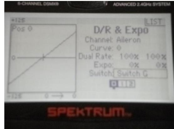
Picture 4. Next, physically move the switch to position 1 (center) and the screen should look as shown. The center position 1 should be highlighted and curve 1. This is snap roll rate, for me. I normally use more aileron to snap roll. Also notice the increase in expo to correspond with the extra throw. This allows the plane to feel the same around neutral stick when flying, with most extra control reserved for the snap roll maneuver itself.
