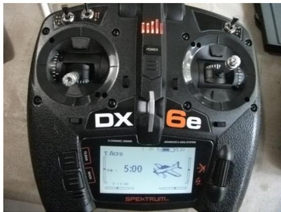
Picture 2. Scroll down to switch and select the switch you want to use to set up your dual rate. I selected switch G because it is a three position switch and I want a single switch to access my snap and spin conditions. With the physical switch position in 0, you notice the 0 is highlighted and the 1 and 2 are not. It also shows curve 0. This is the default.
